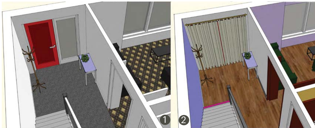
29 Image 1 shows a typical front door, while Image 2, shows a front door with a curtain drawn over the inside of the door to disguise the exit.
